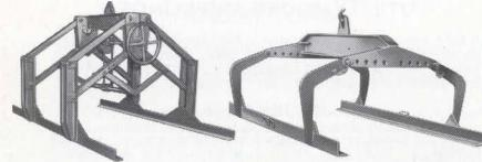
Figure 9-48 SHEET LIFTER — Low headroom type — Easily operated by one man — Suitable for the economical handling of large quantities of material — Adjustable for sheets of various widths — Hand wheel, pendant hand chain or electric motor operated — Capacities to 10 ton.
