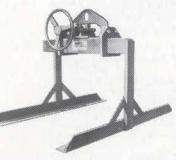
Figure 9-102 PALLET TONG — Suitable for handling paliets, flat panels, sheets, etc. — Hand wheel adjusted for various width material — Capacities to 10 ton.
