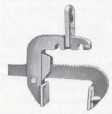
Figure 8-117 RATCHET TONG — Close adjustment to the load over the full range of tong opening — Lifting eye adjustable to balance load — Powerful grip — Suitable for handling boxes, timbers, bars, structural shapes, etc.
