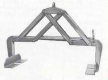
Figure 9-103 PALLET TONG — Semi-automatic — One man operation — Suitable for pallats, panels, cartons, boxes, etc. — Quickly adjusted to various widths — Capacities to 5 ton.
