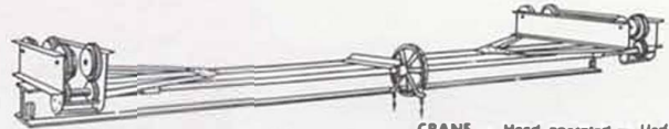
Figure 9-3 CRANE — Hand operated — Underhung — Single girder — Geared wheels and pendant hand chain — Roller brg. — Cap. to 10 ton — Also hand push and double girder types.
