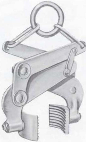
Downs Billet Tongs are designed for handling any type material that needs to be vertically lifted and then lowered horizontally or vice versa. The tongs are of the compound leverage type, which exert a strong positive grip on the load.
