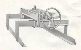
The leg length, "Dimension B" will govern the depth of the stack of sheets which may be picked at each lift and will also govern the overall height of the lifter. Where headroom is a problem, "Dimension B" may be decreased at no additional cost. The desired leg length must than be specified, otherwise they will be shipped as listed.
